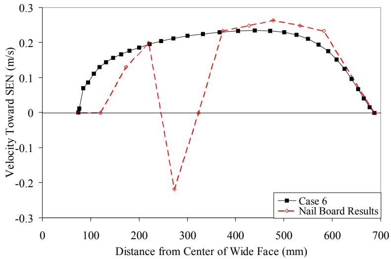
Fig. 8 Comparison of calculated and experimental meniscus velocity
