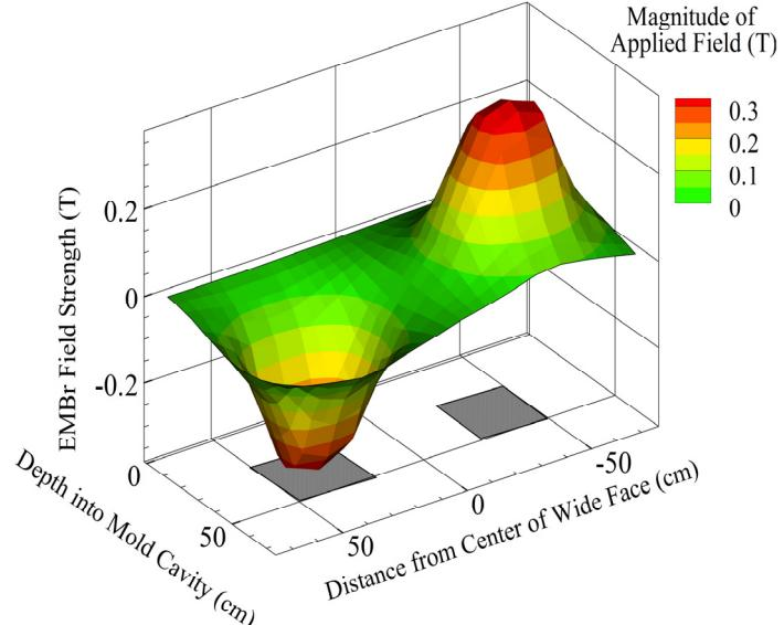
Fig. 2 Measured electromagnetic field contours (0.355T)
