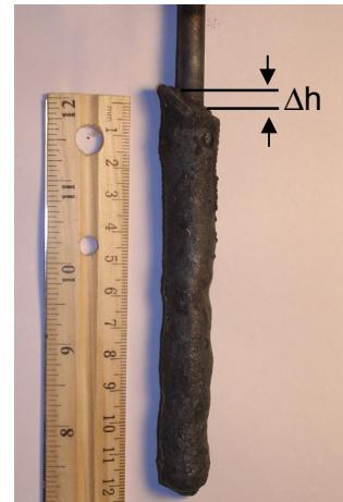
Fig. 6 Nail photo showing measurement of solidified knob
